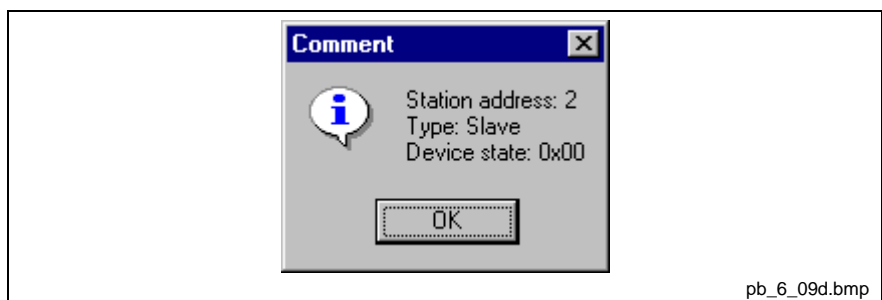
Fig. 8-8: Device type and device status of a slave
